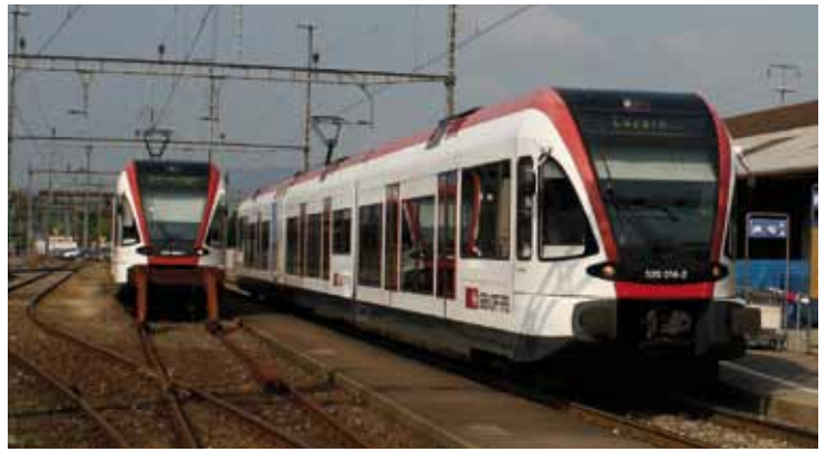
Stadler GTW lightweight articulated three-coach electric multiple units at Lenzburg, Switzerland. These can also be two-coach units for less busy routes. The extra short section, with the pantograph, is the four-wheel drive unit on to which the adjacent coaches are articulated. This can house a diesel motive power unit rather than the electric drive seen here
