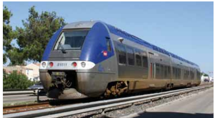
A three-coach diesel multiple unit on a French branch line approaching Aigues-Mortes in Provence. There are several variations of this class including two-coach units
