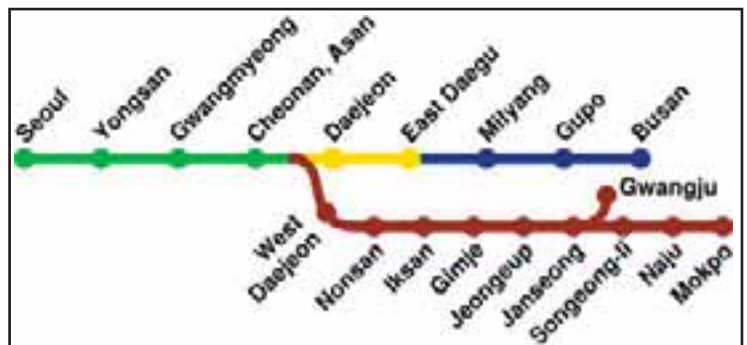
NETWORK DEVELOPMENT: South Korea's shared track is in green, 186mph line in yellow. The classic track in dark blue and red will be mostly upgraded within the next three years
