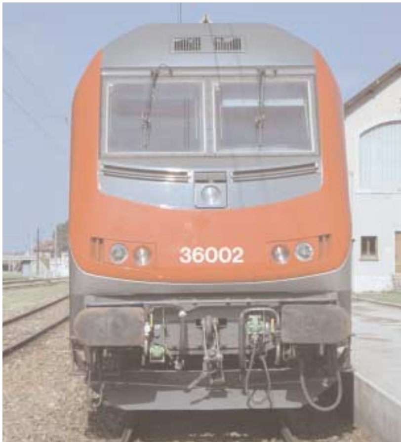
Coming soon to a line near you? European railways may soon be able to run trains into Britain. This French electric locomotive runs on 1.5kV, 3kV (as used in Belgium and Italy) and 25kV (as used in parts of Britain). It already works between Calais and Italy, picking up Channel Tunnel freight hauled between Calais and Willesden by British locomotives
