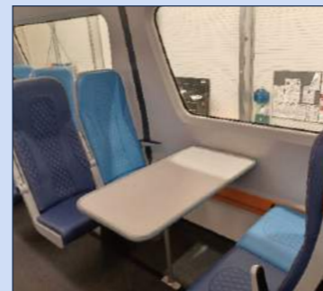
Interior of the prototype Revolution VLR vehicle at Ironbridge. Interior fit-out is configurable to various requirements and can include toilets. As fitted out, seats face towards a single table-bay on each side in the middle of the vehicle. All the forward-facing seats are in the rear half of the car in either direction of travel. We wonder whether this will result in unbalanced loadings, as most passengers prefer to face forwards!
