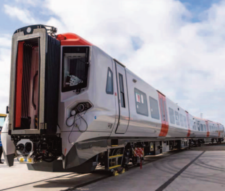
TESTING: The first of the Civity class 197 diesel trains began test running in May. They are expected to enter service next year. The bodyshells were built at CAF's Beasain plant in Spain with final assembly at the new £30 million Llanwern factory near Newport, south Wales, where 200 people now work.
