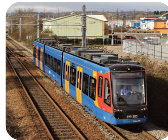
TRAIN: On Network Rail territory, a tram-train approaches the Rotherham terminus at Parkgate. Note the white, raised check-rails on the crossover
