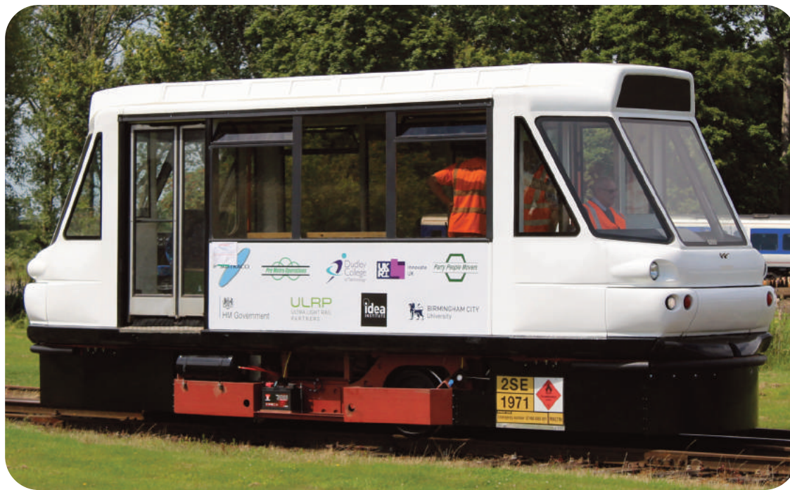
LIGHT FANTASTIC: Fuelled by biomethane, the ultra light railcar in action at Long Marston
