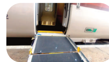
New-style ramps were needed for LNER's Azuma trains. The ramps are stored on the platform and staff are required to help wheelchair users
