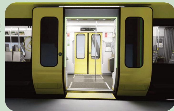
GAP GONE: The Merseytravel train with retractable boarding ramp safely bridges the space between train and platform
