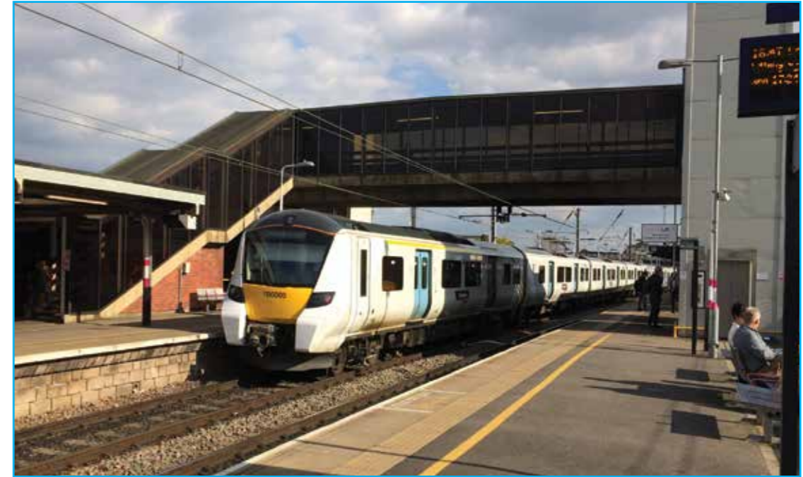
BEDFORD: A new Siemens-built class 700 train emphasises how electrification 35 years ago transformed the Bedford-London service. The BedPan catenary was designed for suburban services and may have to be upgraded once the Midland to Derby, Sheffield and Nottingham line is electrified for higher speed inter-city trains.
