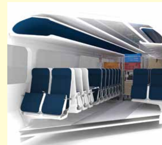
The system has been designed to work on running rails that are fitted to the existing seat rails. All the mechanisms are fitted within the void between the rails
