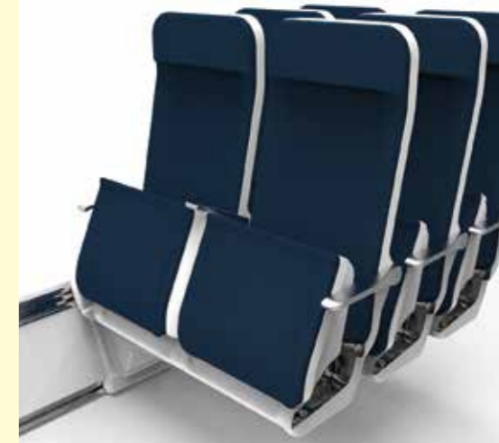
The mechanism allows any rubbish left on seats to be tipped on to the floor for easier cleaning after the seats have been stowed and without compromising passenger comfort
