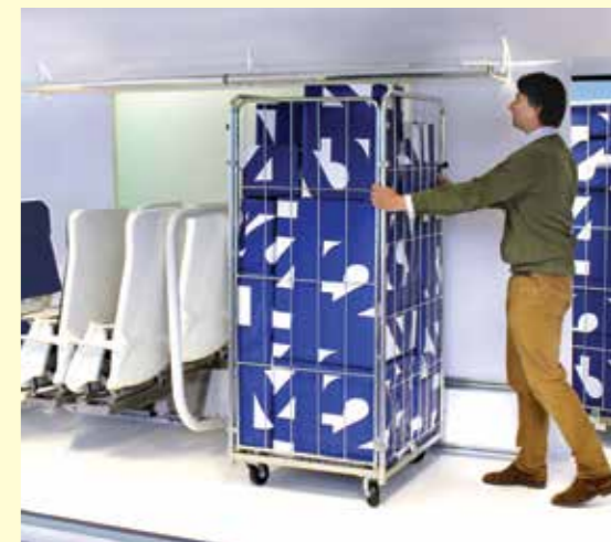
The system allows seats and tables within the carriage to be automatically stowed to create space for high value cargo including deliveries from online retailers or fresh foods
