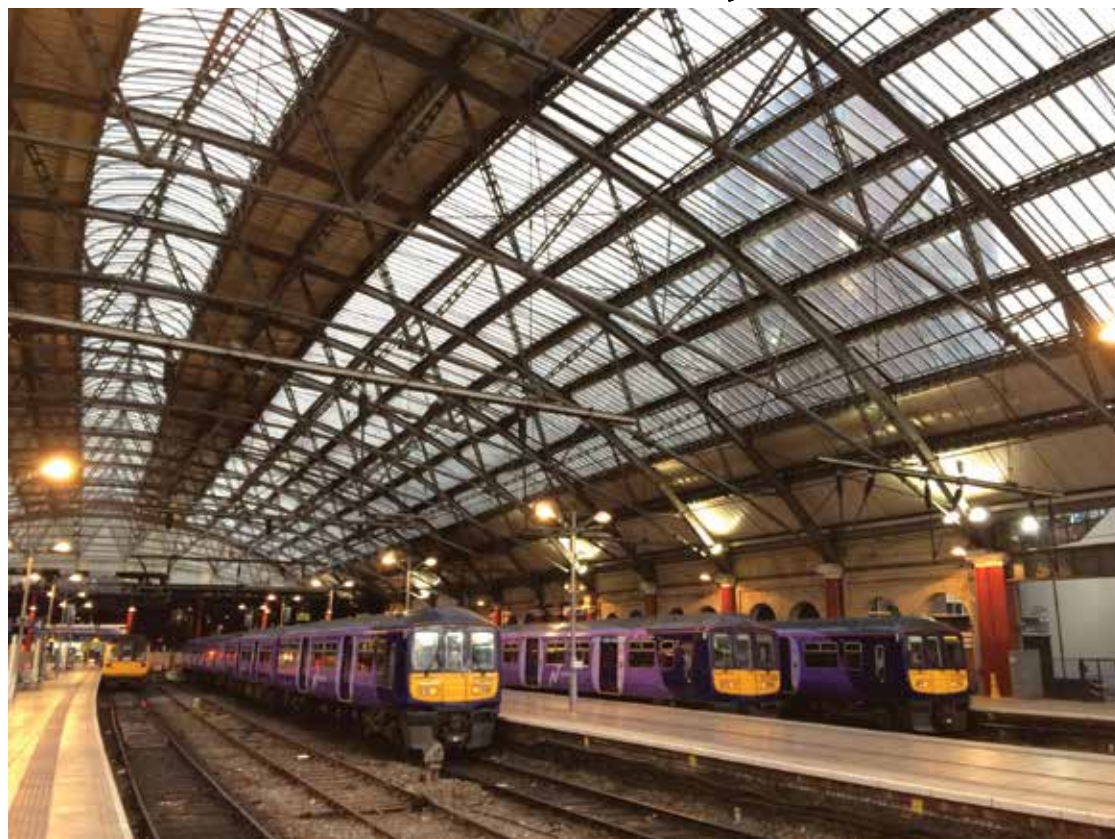
THE BENEFITS OF ELECTRIFICATION: Three electric former Thameslink trains at Liverpool Lime Street with a Pacer on the left. The 319s are already providing more capacity and comfort for passengers travelling from Liverpool to Wigan and Preston. As electrification spreads across the north west of England, more of the unloved diesel-powered Pacers will be displaced
