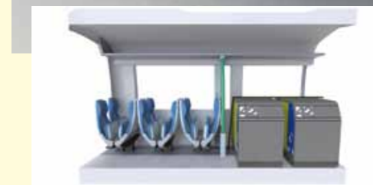
CARRIAGE: 42 Technology's new design allows freight and passengers to be accommodated
