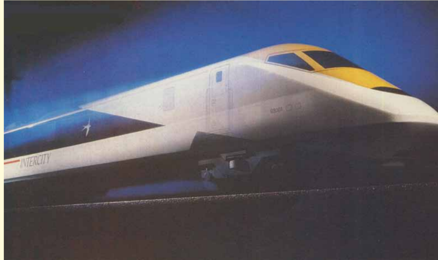
BRITISH RAIL'S IC250 TRAIN CONCEPT: This was one of the projects that got lost in the rush to privatisation more than 20 years ago. It would have delivered a non-tilting inter-city train that could run at speeds up to 155 mph on the West Coast main line, but major track realignment and increased cant on many of the line's curves would have been required
