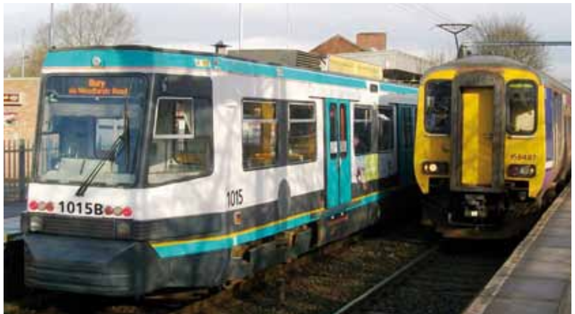
A Manchester Metrolink tram and a Sprinter diesel train sharing Navigation Road station near Altrincham which is split into two single tracks, though both are controlled by Network Rail's Deansgate Junction signal box. Bosses at Transport for Greater Manchester have already said they would like Metrolink services to use the rail network to reach more towns and suburbs. One possibility is incorporating the Ashburys to Marple line into the Metrolink network
