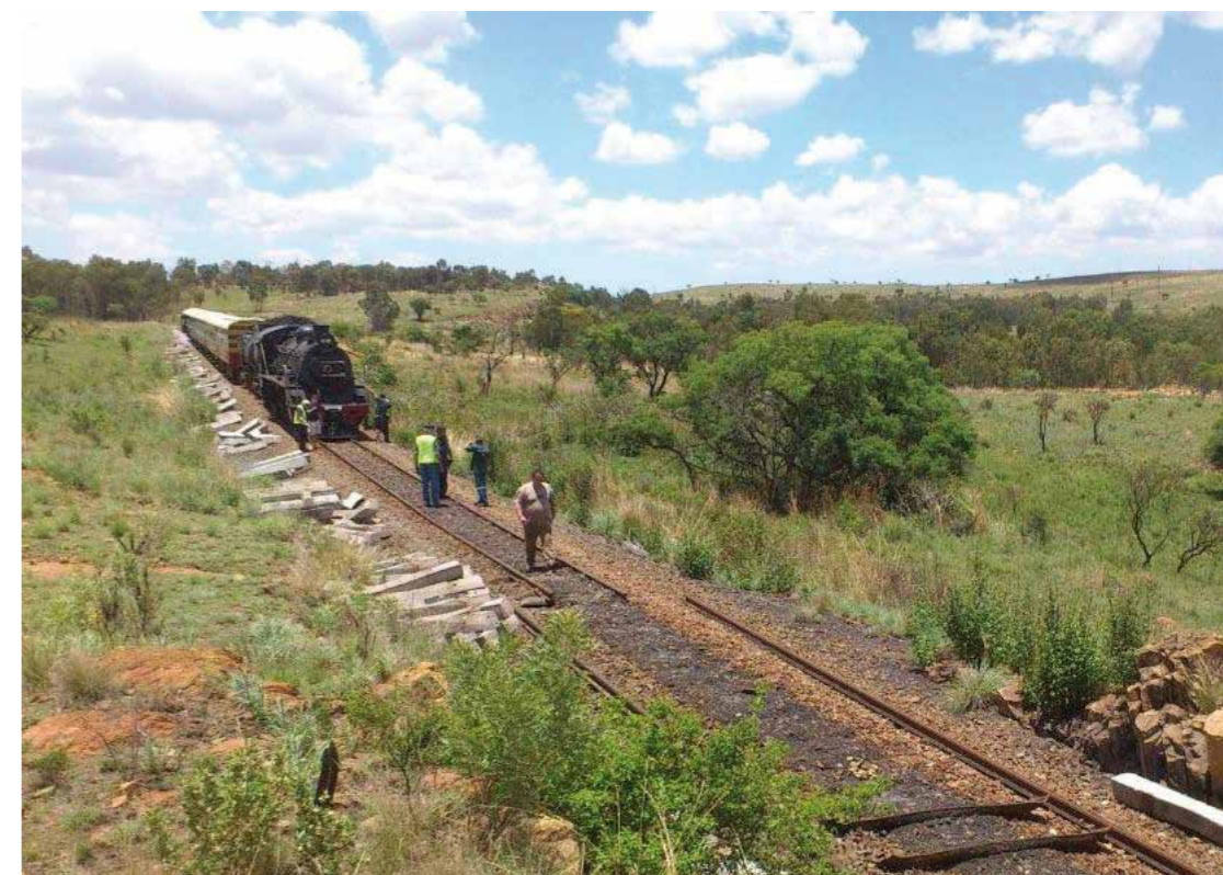
STOP: A steam excursion is halted in the South African bush after steel sleepers were stolen
