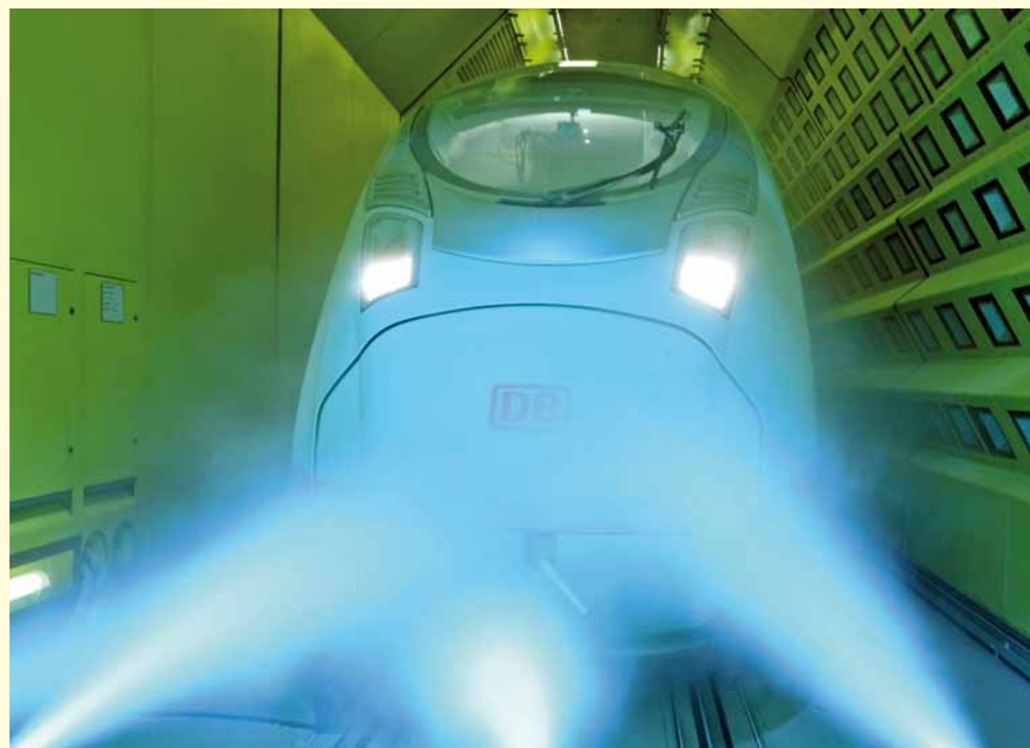
FORGING AHEAD: A Siemens Velaro high-speed train being tested for extreme weather conditions in a wind tunnel at the Rail Tec Arsenal in Vienna. This Velaro was built in Krefeld and will enter service with Deutsche Bahn as an ICE3. Other versions of the train have to operate at 185mph in tropical heat, rain showers and snow storms in Spain, China and Russia
