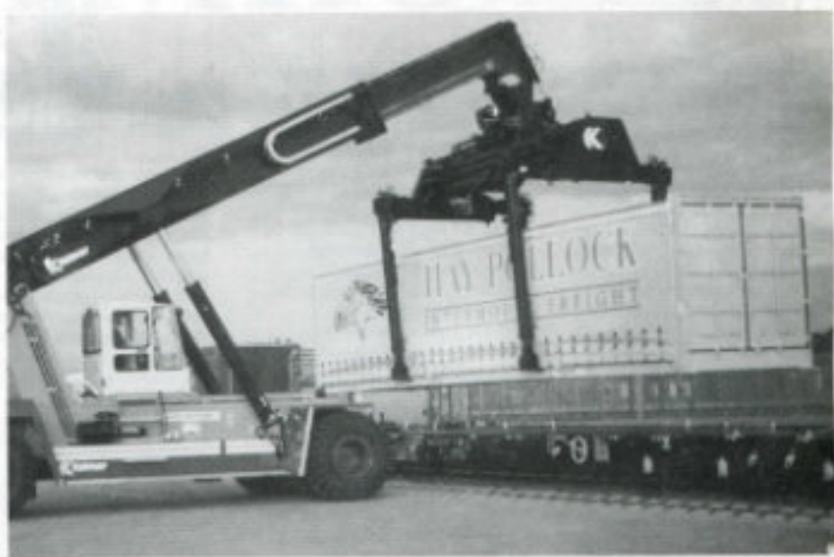
A long way to go: The first British-built 13.5 metre curtain-sided swap body is transferred from a road vehicle to a rail wagon at the Trafford Park exhibition. This is one of 12 to be supplied by European Intermodal Products to international freight company Hay Pallock
