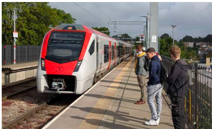
A class 756 Stadler Flirt arrives at Waun-Gron Park in the Fairwater area of Cardiff, taking power from the recently installed overhead wiring
