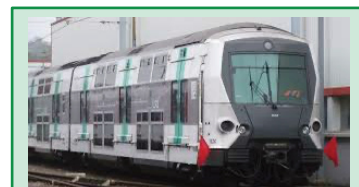
EXAMPLE: The Latest Paris RER train is double-deck but with three entrance doors per car
