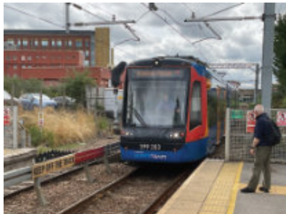
FLEXIBLE INFRASTRUCTURE: A light rail tram train is followed by a heavy freight train within five minutes on the same track at Rotherham. Infrastructure is expensive and its economic benefit needs to be fully exploited
