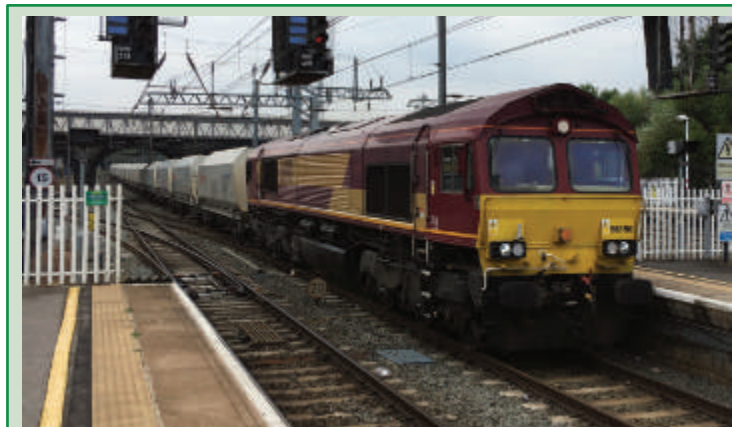
DIESEL POWER: A northbound freight train of aggregate wagons works through Bedford station on the Midland main line, which is already very busy with passenger trains. More will arrive from Oxford with East West Rail in a few years time. Electrification of the Midland main line now extends from London for 82 miles to Market Harborough, as well as to Corby. But to make rail freight work more efficiently, electrification of the Midland main line needs to be completed as soon as possible, as well as many short sections of other lines which would allow many freight trains to switch to more efficient electric haulage Picture: Railwatch
