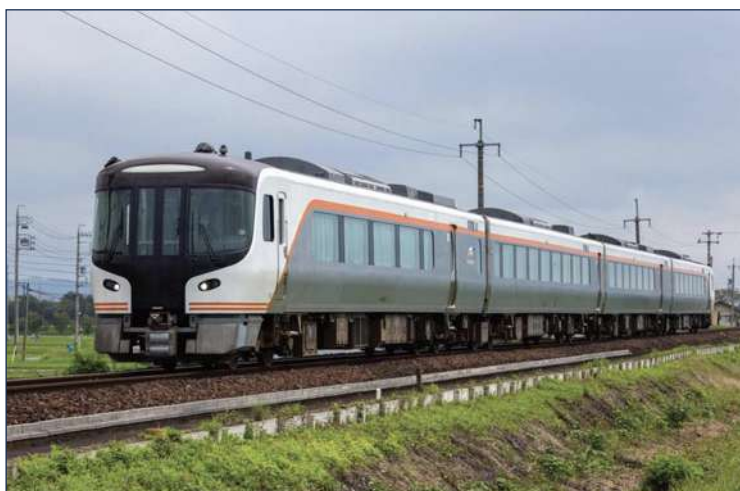
The diesel multiple unit replacement in Japan, the HC85 train
