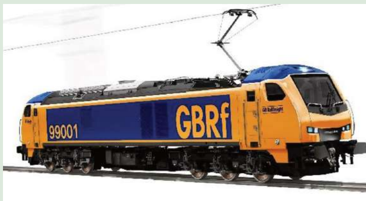
FUTURE PROOFING: The new Stadler heavy freight electric locomotive for GB Railfreight – with a backup diesel engine
