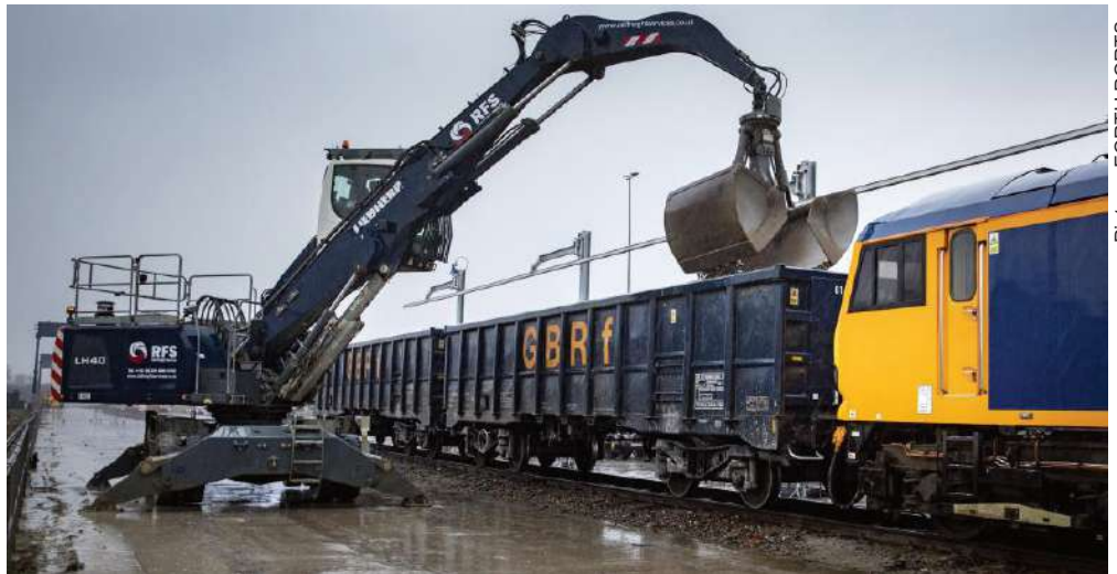
MOVEABLE: The 25kv power supply is retracted to allow cranes space to load trains
