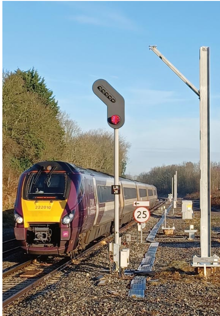
A diesel passenger train nearing the platform at Market Harborough station, past recently installed electrification masts
