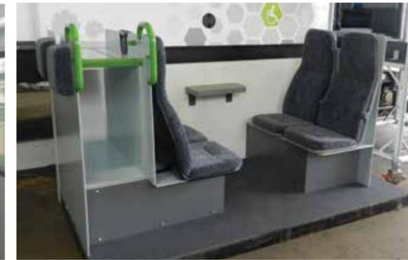
Seat unit and storage, left, specially for a folding bike
