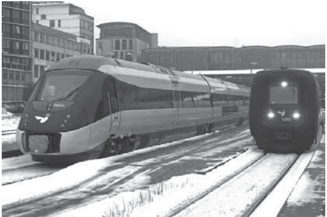
CONTRAST: A new four-car IC4 diesel train, left, which is taking over services from the 1980s-designed IC3 diesel on the Danish route between Arhus and Alborg Picture: Asger Christiansen of Arhus
