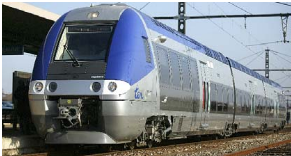
French National Railways has recently awarded Bombardier a £248million contract to build 100 extra AGC high-capacity trains for its regional network. Bombardier is already building 280 of the trains – which have Gresley-style bogies between the coaches – at Crespin in northern France. The trains can run on either diesel fuel, electricity or a combination of the two. Right: Tip-up seats and bike hooks feature in the convertible space. The trains were on show in Lille in March at the international railway industry exhibition
