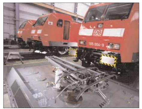
This new locomotive for German Railways is one sign of progress in bringing the railways of Europe together. Makers Adtranz describe it as the first truly European locomotive, being able to operate on 15kV and 25kV systems, through the use of different pantographs.
