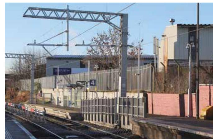
**SPOT THE DIFFERENCE:** Tram-train operation through main line stations is liable to involve the provision of lower platforms to match the lower platforms on the tramway. The difference is shown in this view of the Parkgate-bound tram-train platform at Rotherham Central (platform 4) compared with the main line platform 2 to the right.
